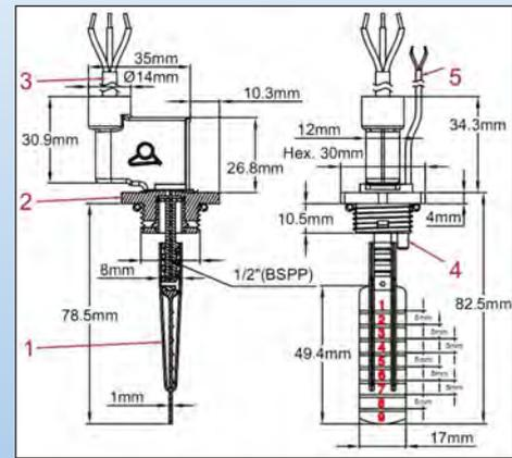
**Main uses:** Water flow detection on water pipes, with simultaneous water temperature measurement
